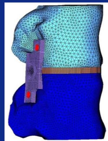
Oblique view of FE model of motion segment with implant
