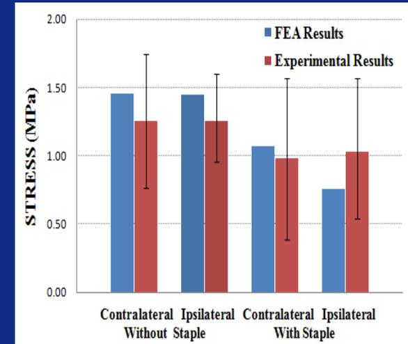
Comparison between FEA and experiments: Stapled model showed lower peak annular stresses and a side-to-side peak stress difference
