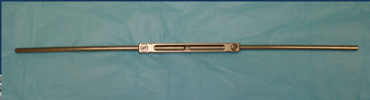
Implantable spinal rod with magnetic actuator
