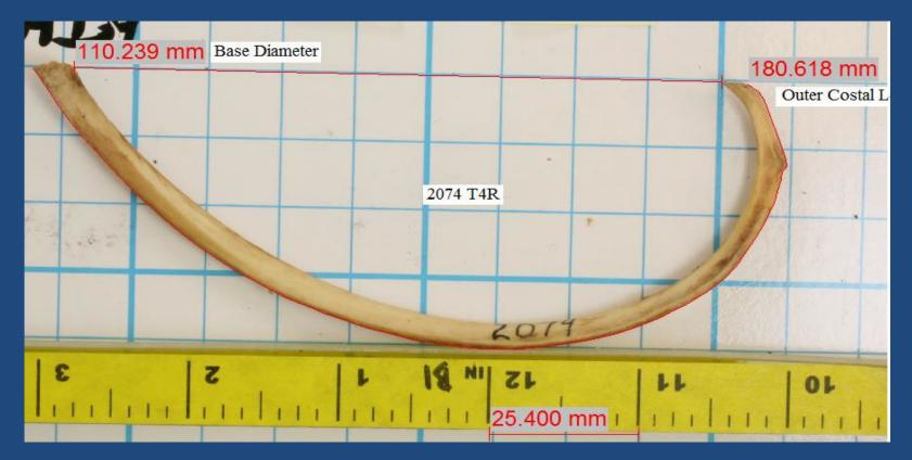
Quantitative measurements were taken with image analysis software. (Scandium Image Analysis Software Olympus, Soft Imaging Solutions)
