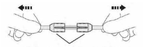
Verify that the collets are firmly attached. The collets should not move back and forth or rotate.
