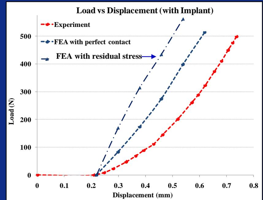
Load displacement curves from FEM with different initial conditions
